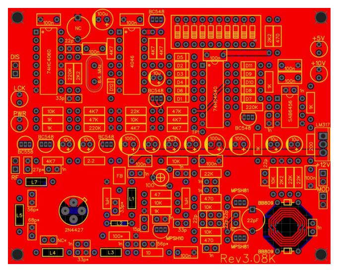
*Important note:* The 10K resistor just at the bottom of the 4046 (between the 22K and 4K7 resistor) should be 2K2.
