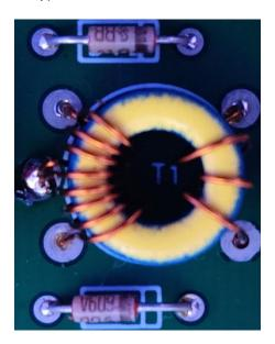
Once you have soldered the toroid in place, re-connect the power and check the following voltages.
